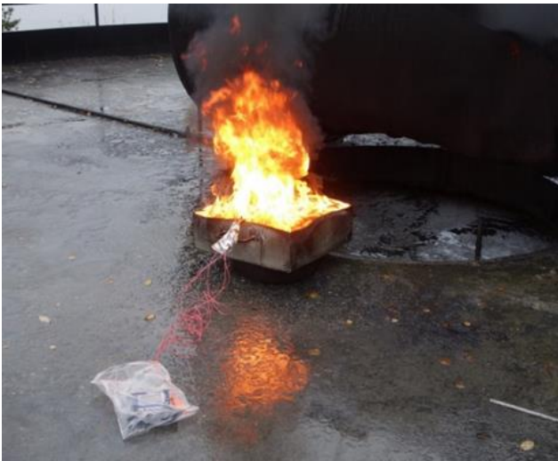
Ignitability / Time before ignitor burn spreads to oil surface
