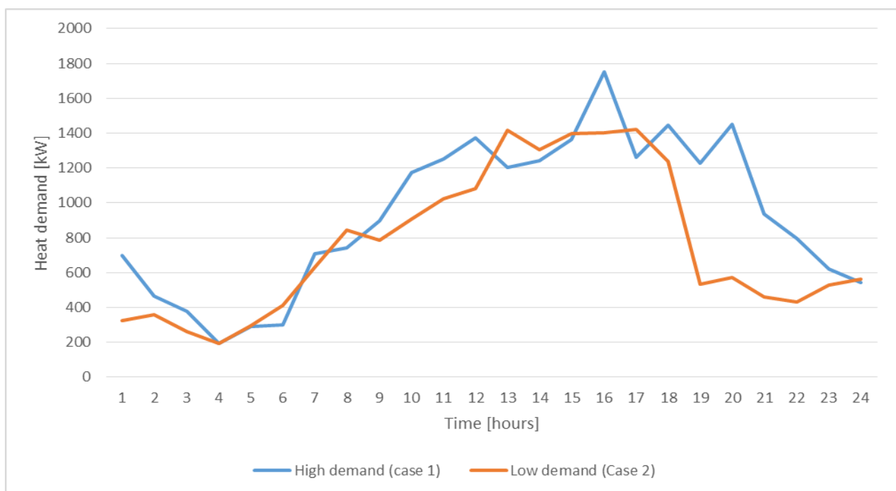
Figure 2. The daily heat demand of two days measured in an industry process: one day with high and one day with low demand
