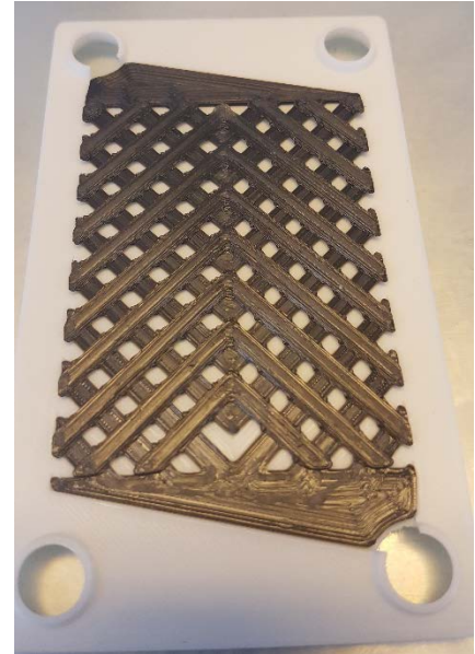
b) Chevron plate with embedded flow pattern
