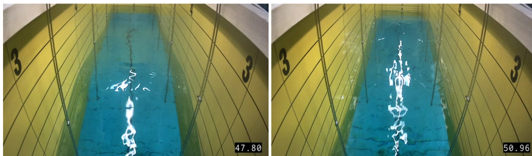
Fig. 17. Two snapshots from video recordings of the moonpool response for MP3 in head sea in regular waves at T = 1.77 s. Dominant excitation of the third longitudinal sloshing mode is observed. See Video 5 for full video of the moonpool oscillations. The time instants are approximately T/2 apart, where T is the wave period.
