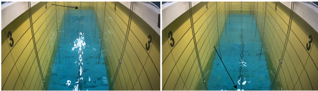
Fig. 12. Two snapshots from video recordings of the piston mode response for MP3 in head sea in regular waves at T = 1.15 s. See Video 3 for full video of the moonpool oscillations. The time instants are approximately T/2 apart, where T is the wave period. The arrows point to the maximum piston mode response in the moonpool.
