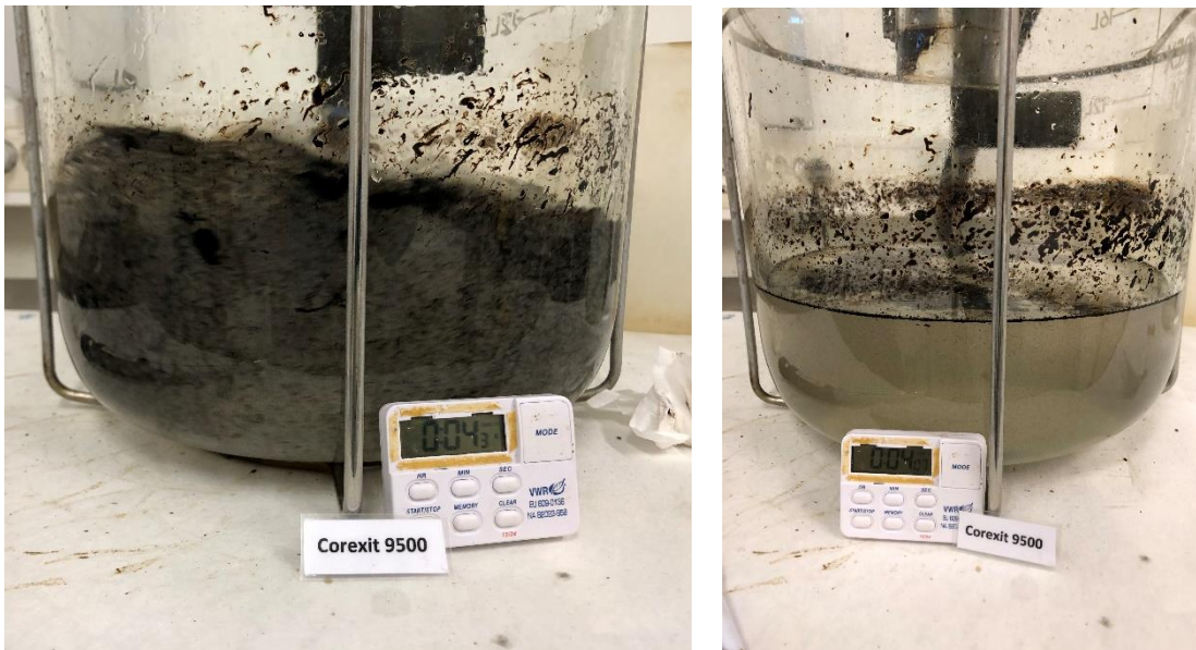
Figure 6-9 MNS test of water-free fresh ULSFO Shell 2019 at 13 °C (Corexit 9500A). Viscosity: 33 564 mPa.s (10s -1 ). DOR 1:25. Left: Dynamic sampling. Right: Static sampling
