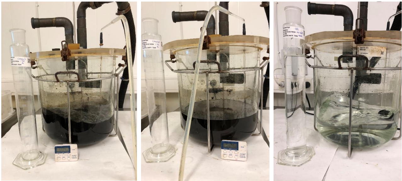
Figure 6-6 VLSFO Shell 2019 (MNS test). Fresh oil (water-free, viscosity 19 450 mPa.s at 10s -1 , 13 °C) after application of Corexit 9500A (DOR 1:25). Left: Dynamic sampling. Middle: Static sampling, larger droplets/lumps on the surface after 5 min. settling. Right: Fresh oil without dispersant (no-disp.)
