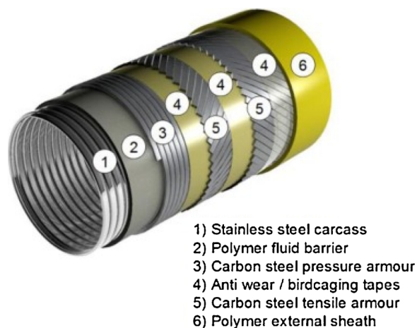
Fig. 9. Cross-section of a typical unbonded flexible pipe Reprinted from (Cornacchia et al., 2019) with the permission from Elsevier.
