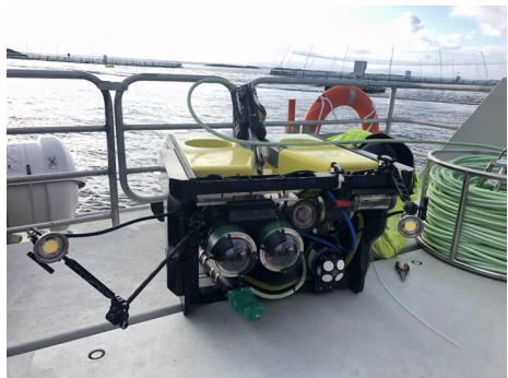
Figure 53: Stereo camera integrated on the ROV
