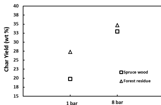
Figure 3: Effects of pressure on spruce wood and forest residue powder charcoal yield
