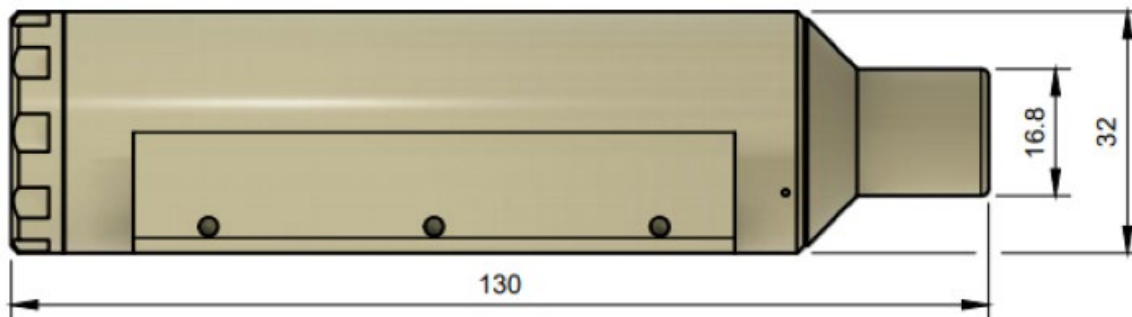
Figure 7 Dimensions WL-21018 Locator-U1 (dimentions are given in mm)
