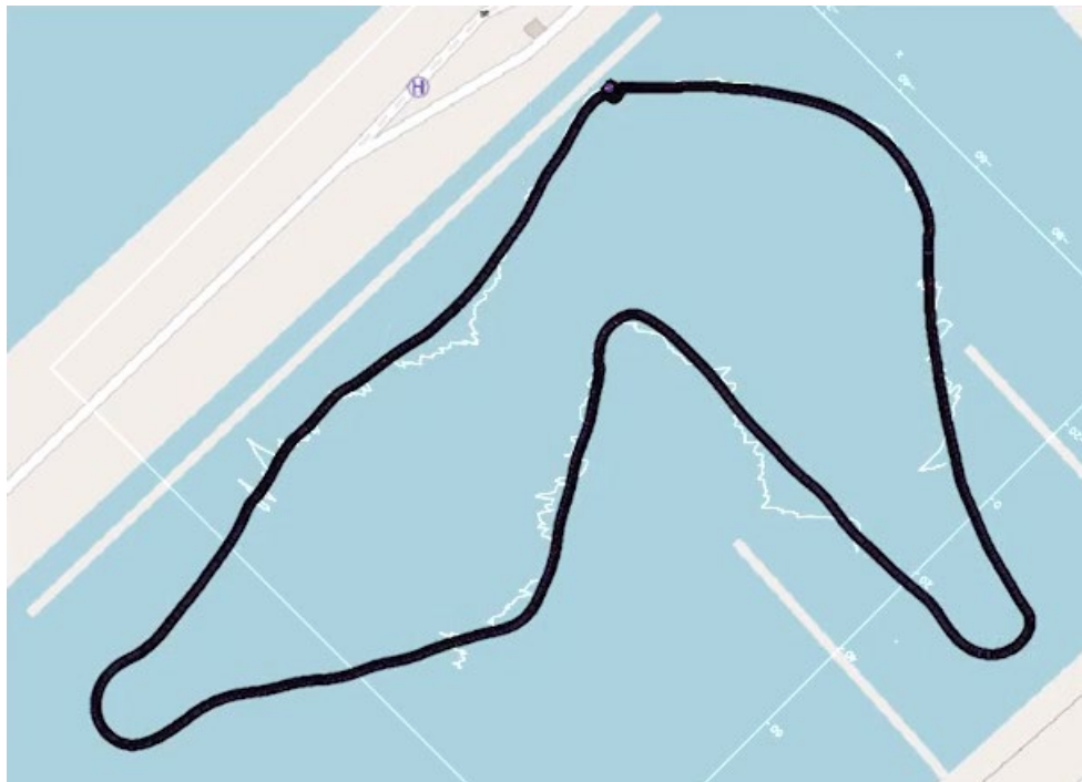
Figure 11 Obtained trajectory and accuracy of the underwater positioning system in Brattøra tests
