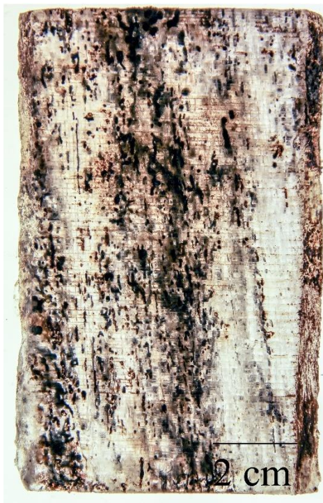
Figure 13 – Vertical thick section at depth (a) 11-22 cm and (b) 22-32 cm at OR+34 for A54-60-c at CRREL. Note how the oil invaded both inter- and intragranular pore space.
