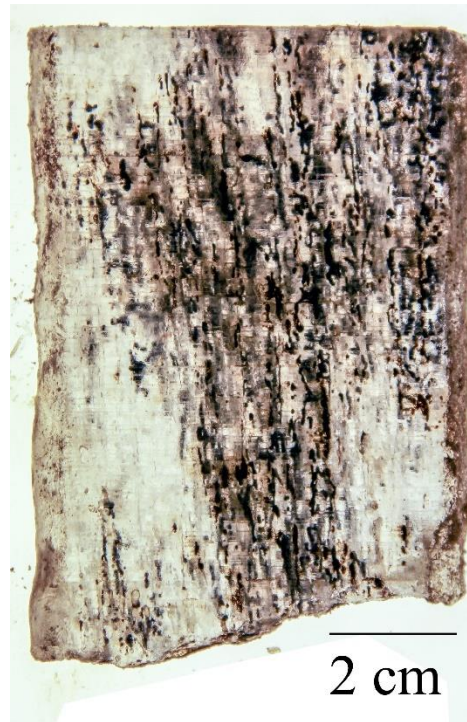
Figure 13 – Vertical thick section at depth (a) 11-22 cm and (b) 22-32 cm at OR+34 for A54-60-c at CRREL. Note how the oil invaded both inter- and intragranular pore space.
