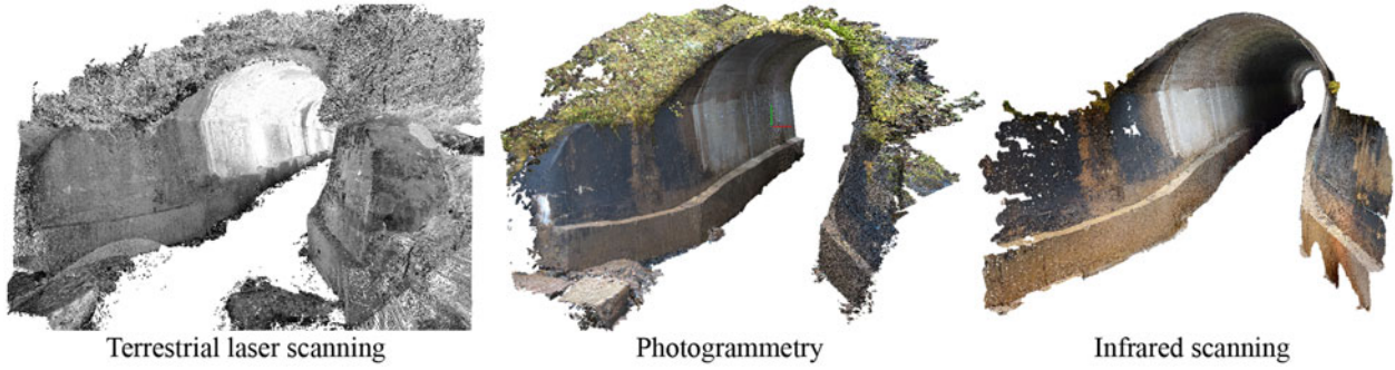
Figure 7. 3D models of Kedkejokk bridge—differences in level of detail between the tested methods.
