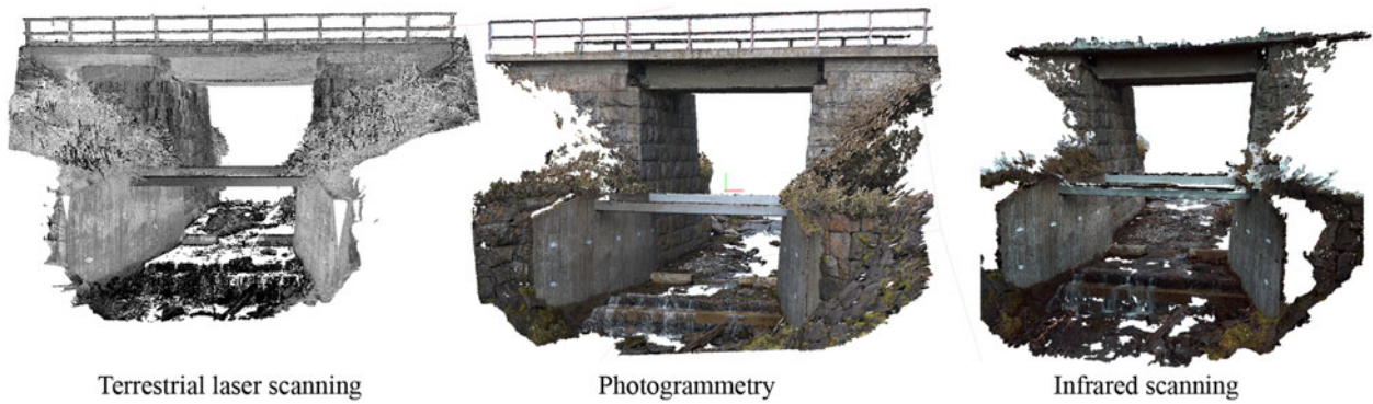
Figure 8. 3D models of Juovajokk bridge—differences in level of detail between the tested methods.
