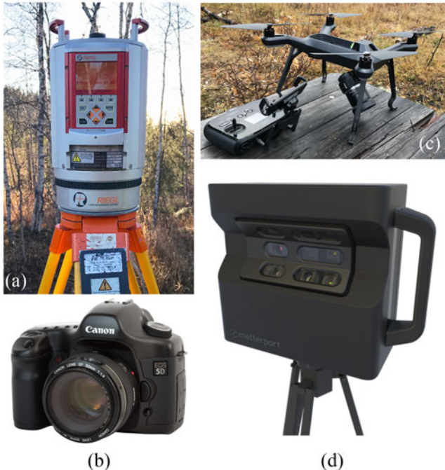
Figure 2. Data acquisition equipment. (a) Terrestrial laser scanning—RIEGL VZ-400, (b) CRP—Canon EOS 5D, (c) unmanned aerial vehicle—3DR Site scan and (d) infrared scanning—Matterport Pro2 3D.
