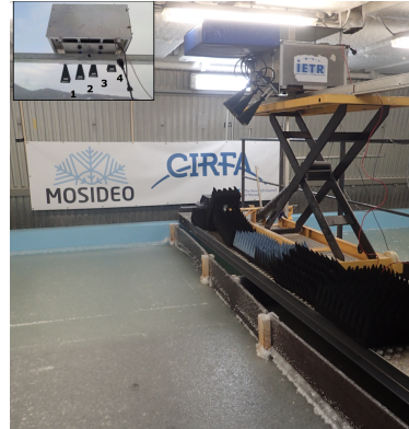
Figure 2: GB-PoSAR set up. Upper left corner shows the alignment of the four horn antennas.
