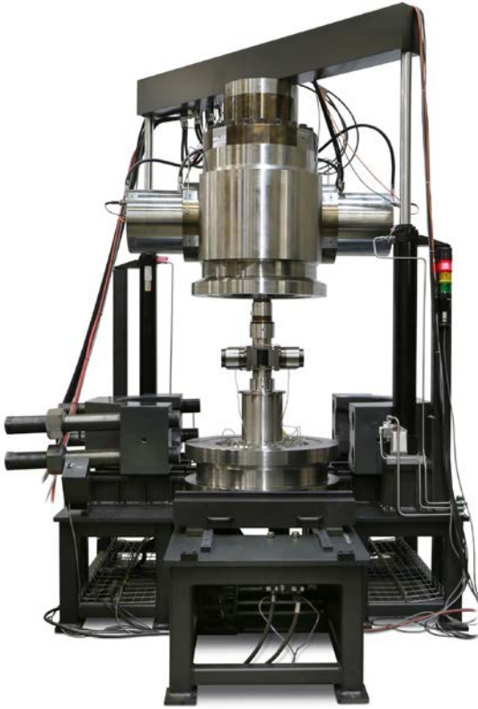
Figure 2. Overview of the true triaxial apparatus, with the dome in the lifted position. The two metal clamps with the threaded rods, for locking and sealing the cell, can also be seen.
