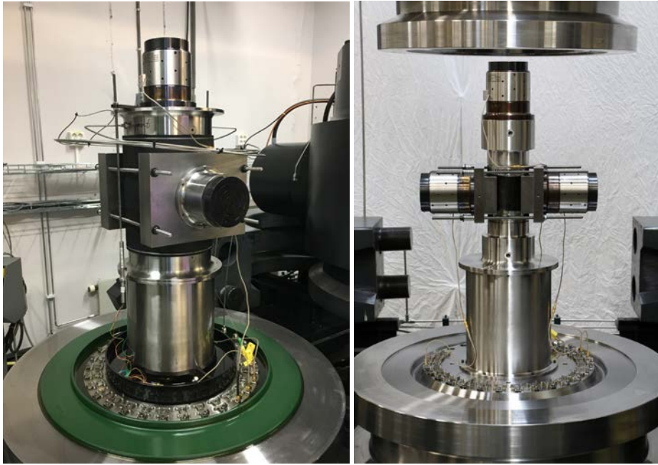
Figure 3. Two different views of the complete sample stack. The rock specimen is located inside the black rubber sleeve, with the axial load cell on top of the stack. The various fluid ports and instrument feed-throughs can be seen on the base flange.
