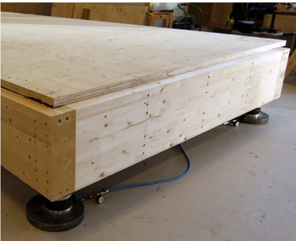
Fig. 3. Free-free boundary conditions: floor element installed on air bellows.
