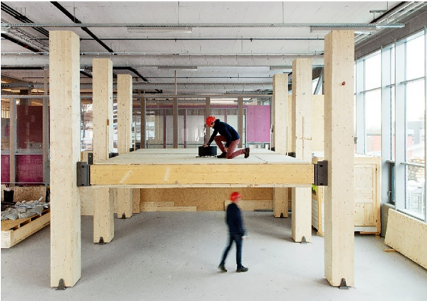
Fig. 2. Woodsol prototype; setup used for the on columns BC measurements, photo: SINTEF/A.-L. Bakken.
