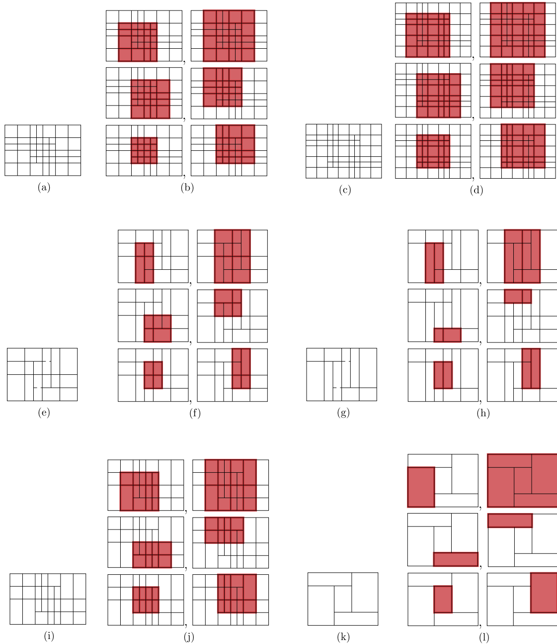
Fig. 15. In (a) an LR-mesh providing MS B-splines of bidegree (3,3) in an equivalent arrangement of the MS B-splines of bidegree (2,2) on the mesh in Fig. 4(a). In (b) are shown the supports of the six B-splines in the linear dependence relation. In (c)-(d) the same for bidegree (4,4). In (e)-(f) we have the same for bidegree (1,1). Note that we have used two extensions (dashed meshlines) to obtain an equivalent arrangement as for the other bidegrees. In (g)-(h) and (i)-(j) we show the equivalent configuration for bidegrees (1,0) and (3,1). Finally, in (k)-(l) we have a comparable arrangement for bidegree (0,0). However, the mesh in (k) is not an LR-mesh.
