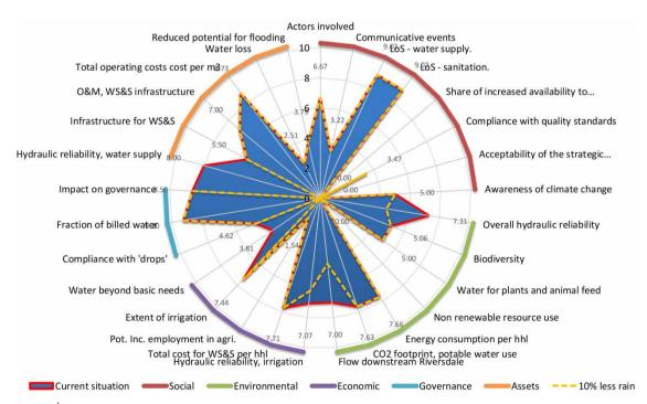
Figure 3 | Spider diagram with results for Riversdale, normalised to a scale of 0–10: current situation and expected future situation if no adaptation measures are implemented and the available water resources decrease due to 10% less rain.
