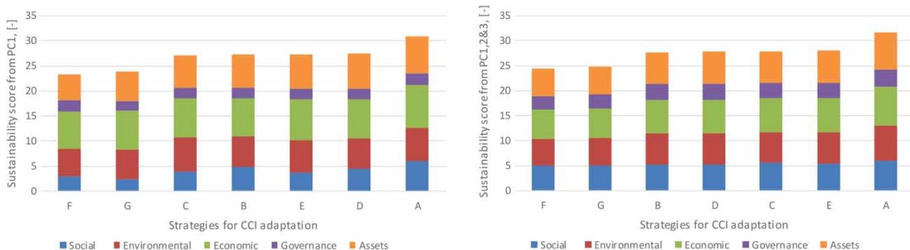
Figure 4 | Comparison of alternatives in Riversdale including the relative contribution to the sustainability score calculated with PC1 (left) and with PC1, PC2 and PC3 (right).
