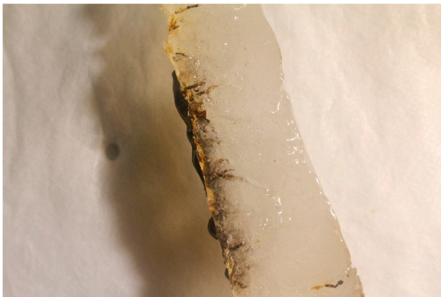
Fig. 16. Illustration of oil filling the cracks and cavities on the cold sea ice.
