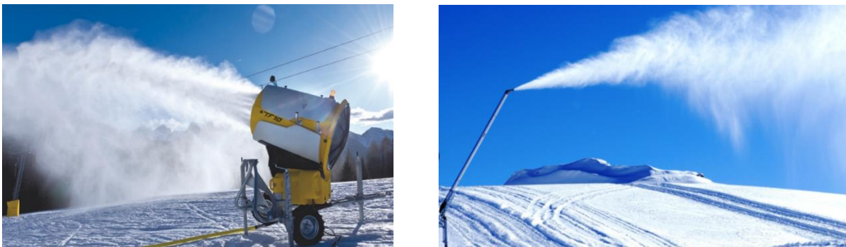
Figure 3: TechnoAlpin's TF10 Fan gun (left) and Borax lance (right) (TechnoAlpin.com 2017). Used with permission from TechnoAlpin.
