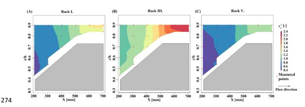
Fig. 3. Interpolated velocity fields at the entrance of the bypass section for (A) rack I, (B) rack III and (C) rack V. The interpolation is based on the normalized resultant velocities ( $v^*$ ); each locations where the filtered ADV data were valid are presented on the figures (red dots).
