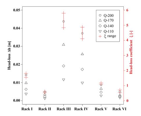
Fig. 2. Head-loss values (m) under different flow rates from 0.110 up to 0.200 m<sup>3</sup> s<sup>-1</sup> for
