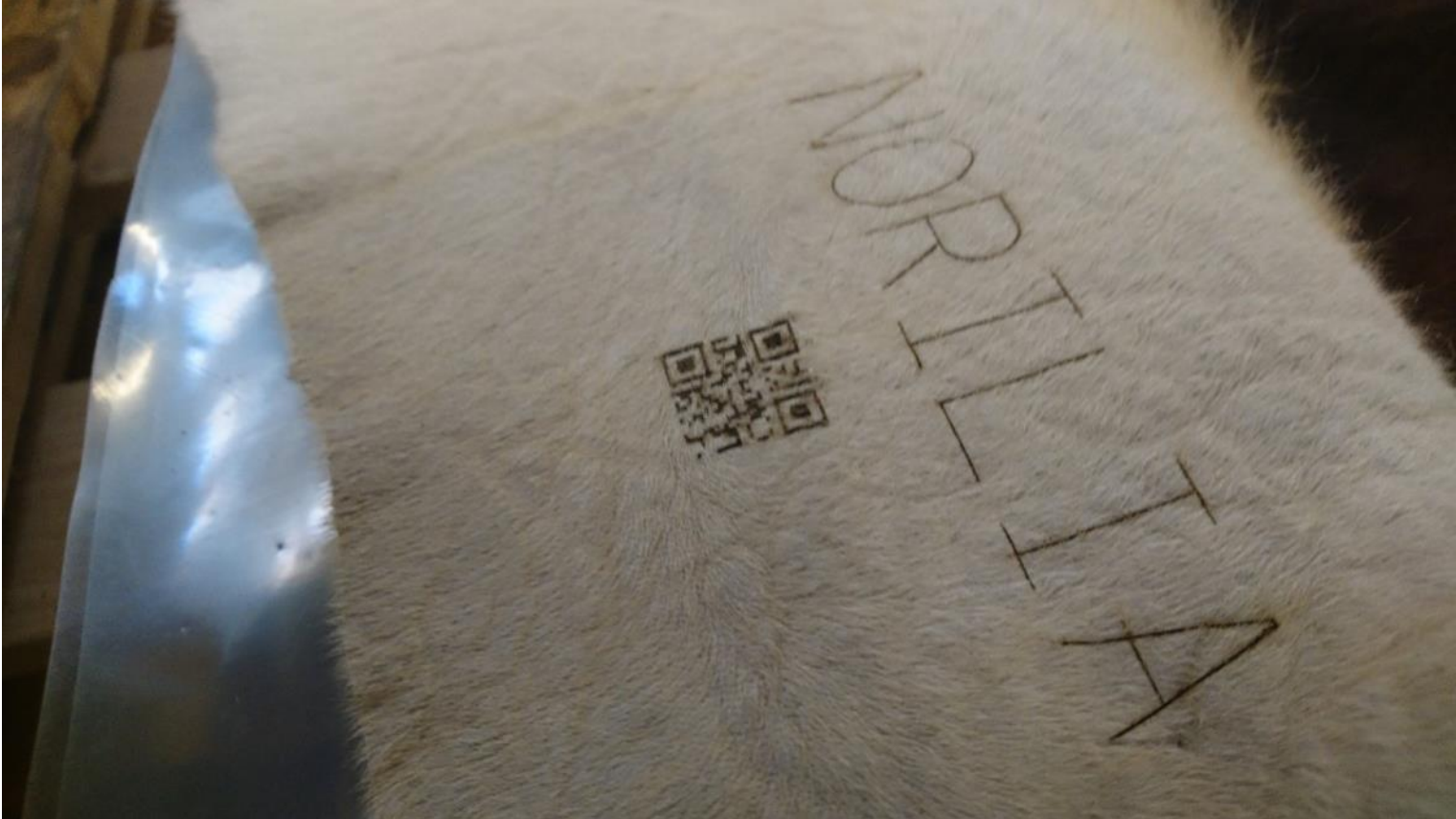
Figure 2: Example of laser tagged hide from tests done in collaboration with Norilia.
