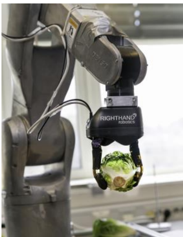
Figure 1: A close-up image of an autonomous robotic grasping of lettuce based on our multi-modal (visual-tactile) robot LfD learning policy.
