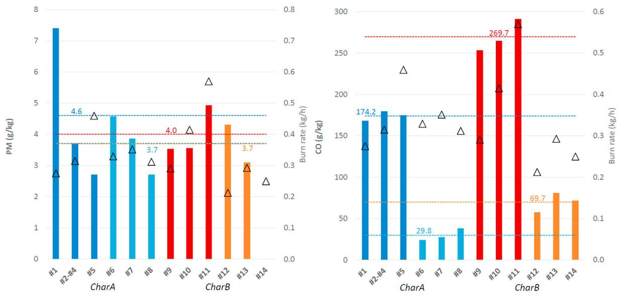
Figure 2: Total PM emissions measured (left, left y-axis) and CO emissions (right, left y-axis) in flue gas and corresponding burn rates (triangles, right y-axis) for all tests. Averaged total PM and CO emissions for each type of charcoal are displayed by the dash lines.
