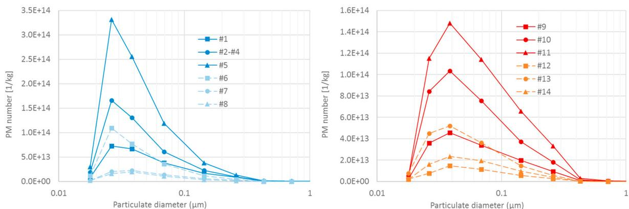
Figure 3: Particulate matter size distribution in particles number per kg of dry charcoal for CharA (left) and CharB (right). Results for tests without catalytic converter are displayed by solid lines, while those with catalytic converter are shown by dash lines.
