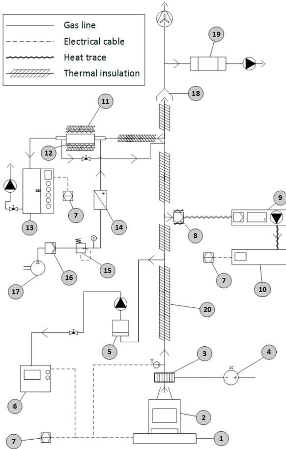
Figure 1: Schematic of the experimental setup. 1. Weight scale; 2. Modern wood stove; 3. Activated catalytic converter; 4. DC power supply; 5. Conventional filter; 6. Servomex online gas analyser; 7. Data collection; 8. Heated probe; 9. FTIR Sampling system; 10. FTIR gas analyser; 11. Heated jacket; 12. Sample gas diluter; 13. ELPI; 14. Air heater; 15. Pressure regulator; 16. Dust filter; 17. Pressurised air; 18. FFDT; 19. Total PM filter; 20. Stovepipe.
