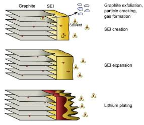
Figure 1: Ageing effects on Li-ion battery negative electrode [2]
