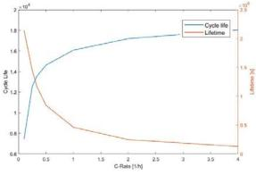
Figure 4: Cell's cycle life versus the c-rate, DOD = 40%,  $SOC_{avg} = 70\%$
