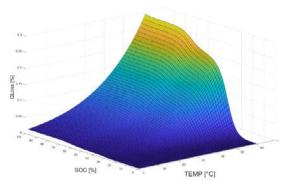
Figure 2: Capacity fade during one hour under idle conditiions
