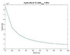
Figure 3: Cell's cycle life versus DOD
