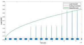
Figure 5: Example of shaving failure due to ageing
