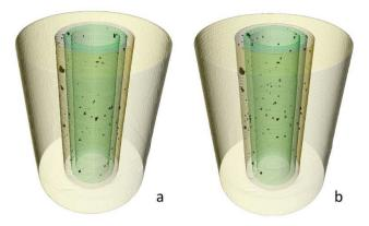
Fig. 3. 3D visualization of CT data from the specimen (a) before and (b) after 20 thermal cycles. Sample diameter and height was about 20 cm. The dark dots in the green cement sheath are defects. The sample is not strongly affected by the thermal cycling.
