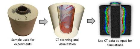
Fig. 7. An illustration of how samples used in experiments were first CT scanned, then reconstructed in 3D (including all defects), and finally used as input in numerical simulations of stress/stain effects.
