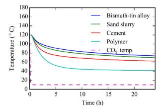
Fig. 8. Temperature at the casing/sealant interface as a function of time while injecting CO2 at 10°C.
