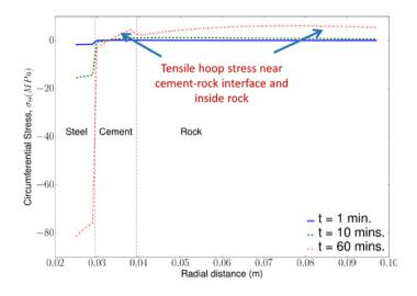
Fig. 5. Circumferential stress profiles as a function of radial distance for heating at 1°C/min.
