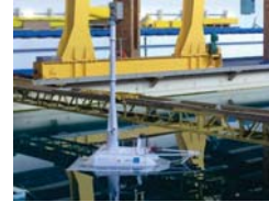
Characterization tests: decay; tilt; pull out
