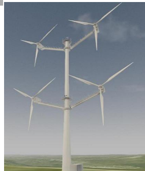
Vestas 4-rotor demonstrator turbine. Source: Vestas ( www.vestas.com )
