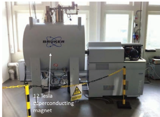
Fig. 1 12 Tesla FT-ICR-MS ultrahigh resolution mass spectrometric instrument
