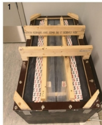
Fixing of the different samples to the airtight box.
