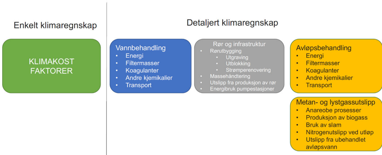
Figure 5.8 Components included in the GHG emissions accounting in the water sector (Borg, 2018)
