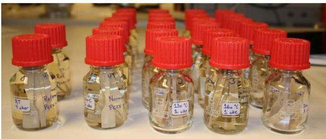
Figure 1. Bottles used for ageing of PEEK with a solid to oil ratio 1:25.
