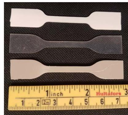
Figure 2. Sample geometry for tensile strength experiments for the three-different studied materials epoxy, silicone and PEEK from top to bottom (solid to oil ratio 1:25).
