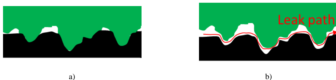
Figure 2. Schematic magnified view of rubber seal surface (black) in contact with a rigid counter surface: a) at ambient temperature; b) rigid surface lift-off and leakage at low temperatures
