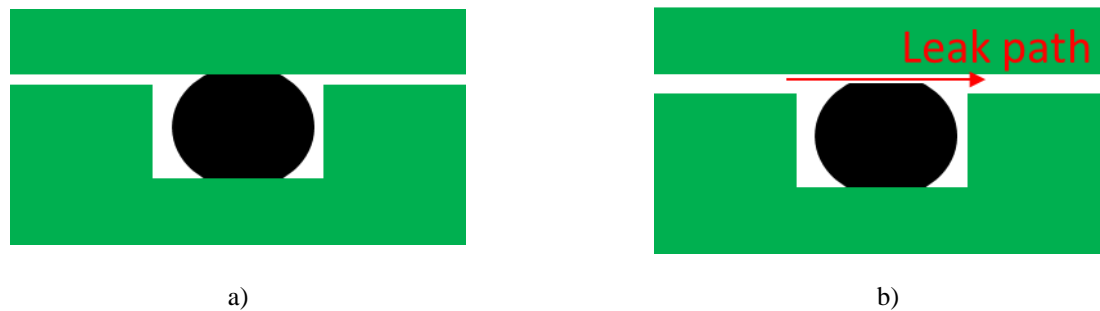
Figure 1. Schematic of compressed O-ring seal (black) in a flange: a) at ambient temperature; b) upper part lift-off at low temperature and leakage due to “frozen” seal
