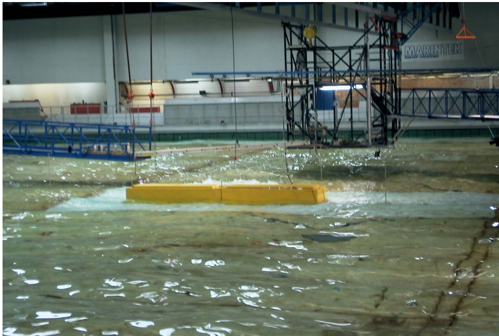
Figure 10: Testing of LNG terminal in shallow water (MARINTEK).
