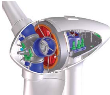
Figure 9. Schematic of Enercon 2 MW wind turbine. (Copy from www.enercon.de )
