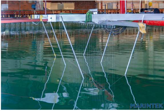
Fig. 4. Wave harp as installed during wave calibration.
