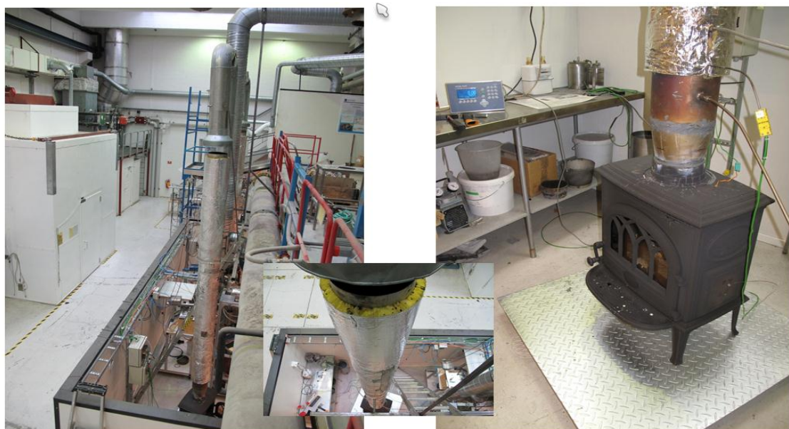
Figure 8. Illustration of experimental setup according to NS3058/NS3059
