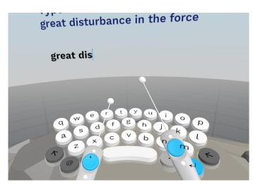
**Figure 1.** The drum-like VR keyboard as implemented in this study (video demonstration: http://boletsis.net/vrtext/drum/).
