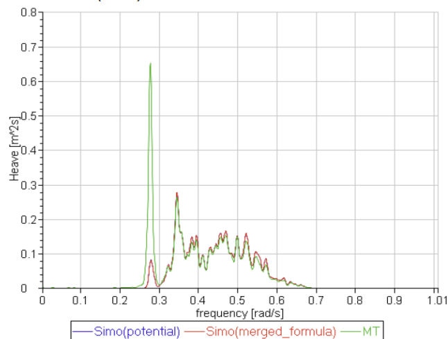
Figure 4: Wave frequency surge spectra (upper graphs) and heave spectra (lower graphs) for seastates 4010 (H s = 2.5 m, T p = 5-25 s) and 4060 (H s = 15 m, T p = 16 s) under head waves and no current. Comparison between model test results (MT), un-calibrated numerical model (Simo(potential)) and calibrated numerical model (Simo(merged_formula)).
