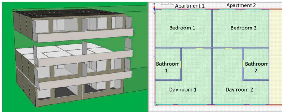
**Figure 1.** Left: Model from 3D-view IDA ICE and right: floor plan for two apartments, each with three zones.
