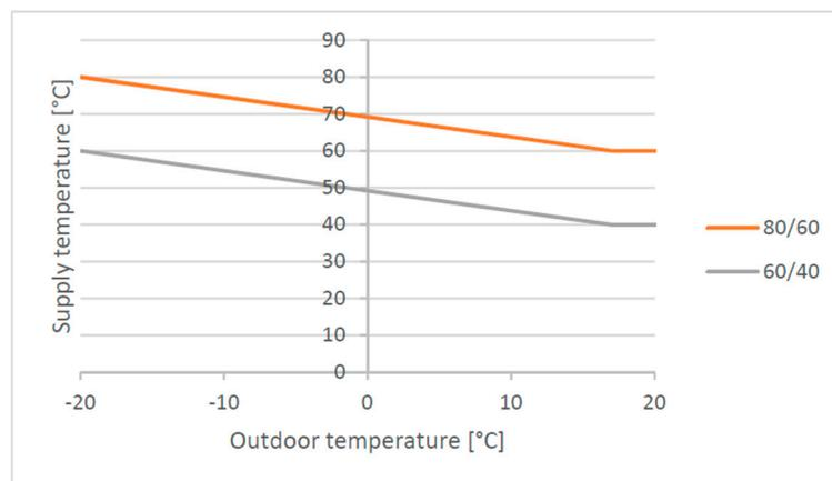
**Figure 2.** Weather compensation curves for the supply temperature of the two radiator systems with dimensioning temperature levels 80/60 and 60/40 °C.
