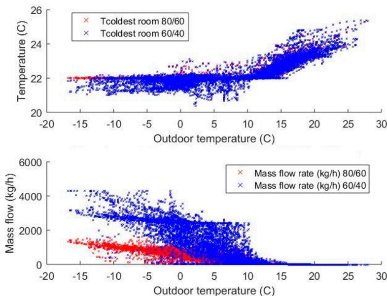
**Figure 6.** Temperature in the coldest room (**top**) and mass flow rates (**bottom**) relative to the outdoor temperature for AB\_03 intermediate renovated.
