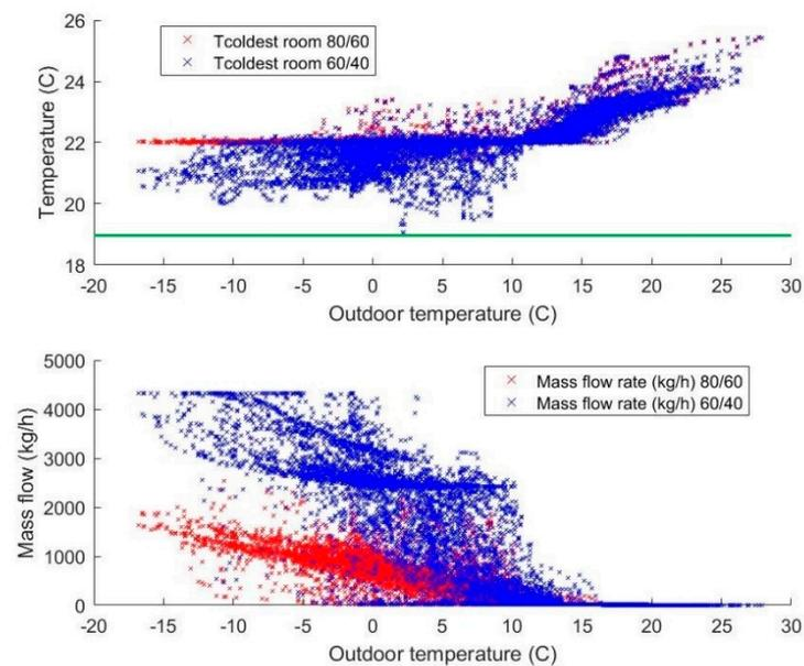
**Figure 4.** Temperature in the coldest room (**top**) and mass flow rates (**bottom**) relative to the outdoor temperature for AB\_03 as-built.
