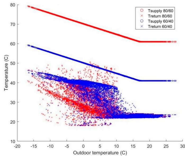
**Figure 3.** Radiator supply and return temperatures relative to outdoor temperature for AB\_03 as-built.
