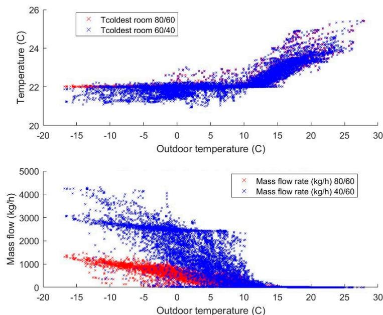
**Figure 8.** Temperature in the coldest room (**top**) and mass flow rates (**bottom**) relative to the outdoor temperature for AB\_03 standard renovated.
