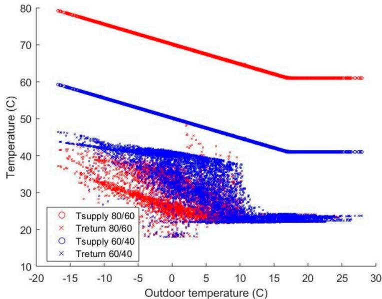
**Figure 5.** Radiator supply and return temperatures relative to outdoor temperature for AB\_03 intermediate renovated.
