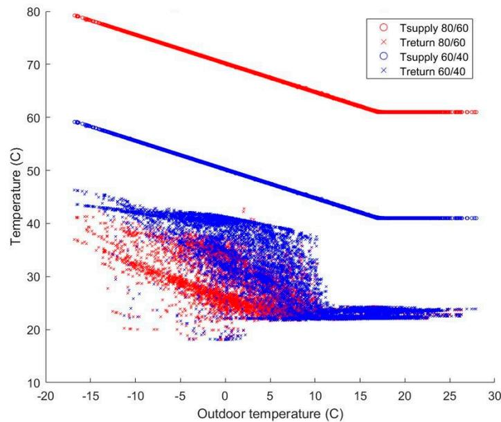
**Figure 7.** Radiator supply and return temperatures relative to outdoor temperature for AB\_03 standard renovated.
