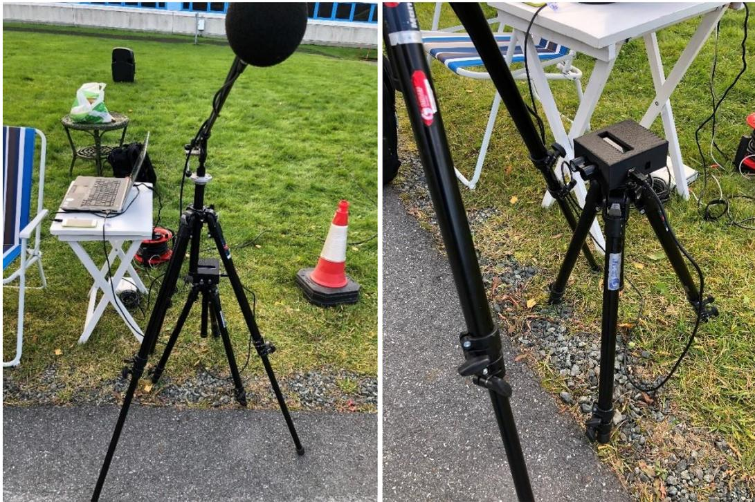
Figure 6. Microphone and loudspeaker (left behind on grass) and Lidar (right)
