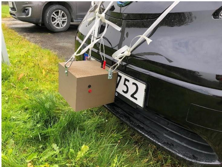
Figure 10. Mounting of loudspeaker for modified AVAS signal
