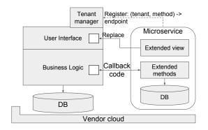
Figure 1: Custom code as intrusive microservices
