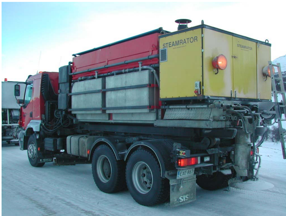
Figur 2.7: Fastsandspreder fra Arctic Machine, NCC Finland
