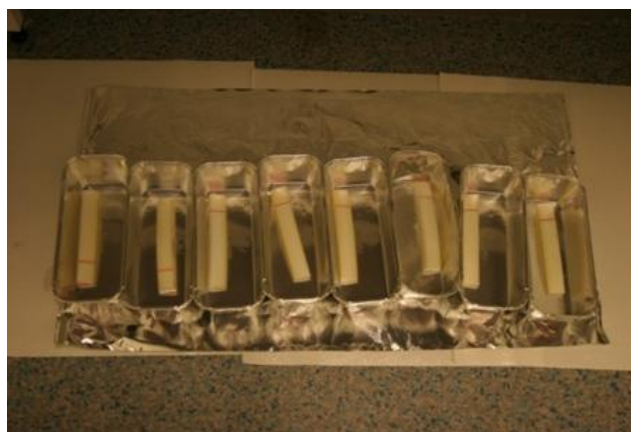
Fig. 3. Bars of disc (2.4 x 15 cm) used for "Dip and withdraw" test
