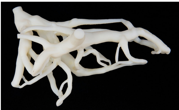
Fig. 12 3D printed liver vascular system using ABS
