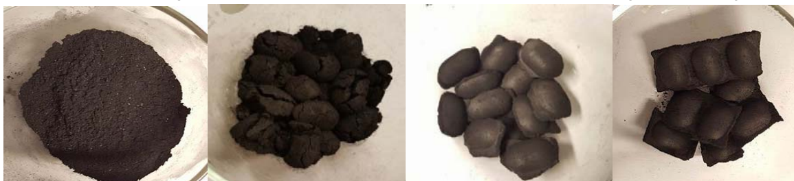
Figure 1: Photo of (a) biocarbon powder, and briquettes made from (b) biocarbon + water 20%, (c) biocarbon + +20% water + 20% alkali lignin and (d) biocarbon + 20% water + 20% starch, after drying at 105 °C for 12 hours
