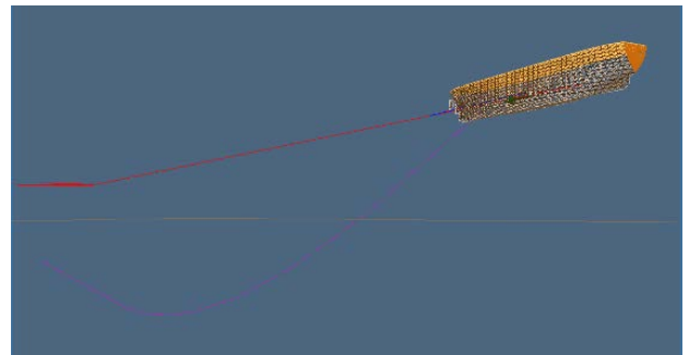
Figure 7. Illustration of simulation model with vessel, and retrieval of crab pot string.
