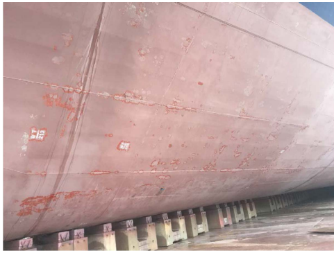
Fig. 3. Damage to the hull painting of Color Fantasy [4].
