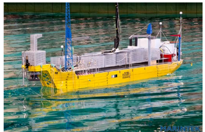
Fig. 1: Photo showing the vessel model in the MARINTEK's Ocean Basin.
