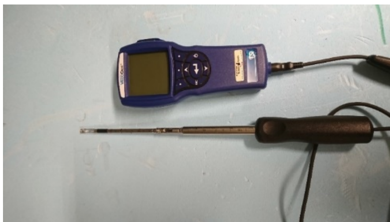
Figure 10 VelociCalc 9565-P along with extendable thermoanemometer probe.
