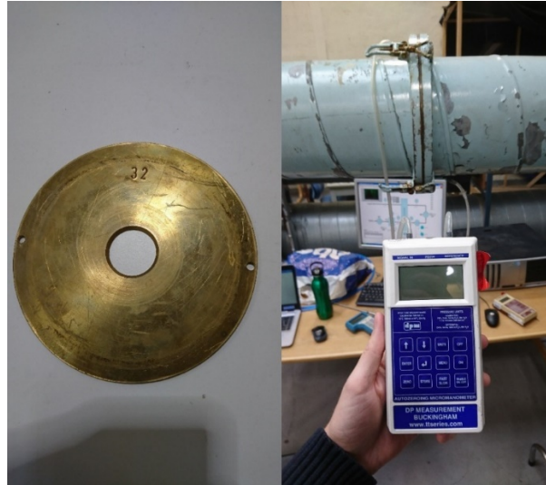
Figure 4 Example of an orifice plate for 100 mm duct with 32 mm opening (left) and lab setup with orifice plate in duct and manometer for measuring the pressure difference (right).
