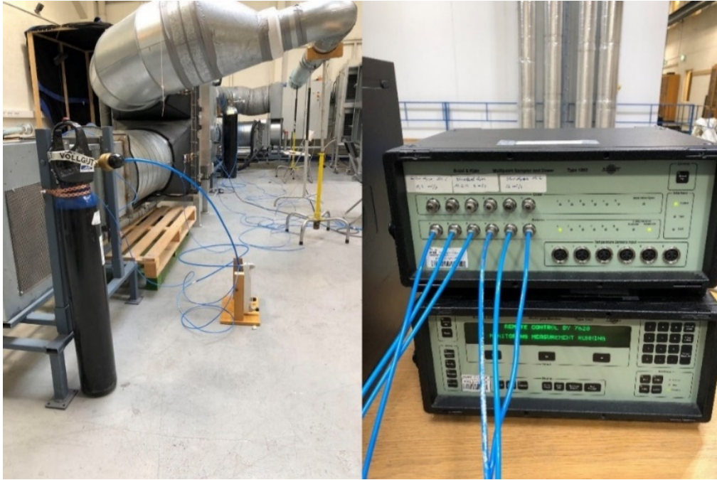
Figure 24 Heat wheel test rig setup: heat wheel and duct with dosing and sampling tubes on the left; the LumaSense tracer gas analyser with sampling tubes.
