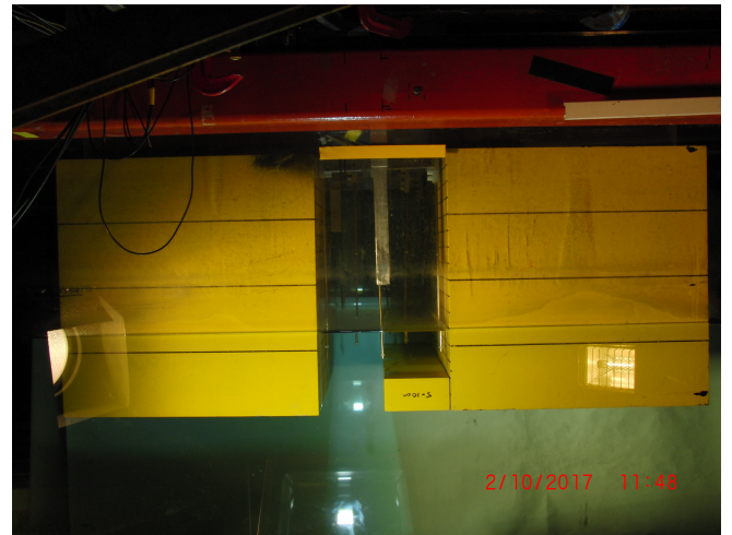
FIGURE 5. EXPERIMENTAL CONFIGURATION (CASE 4) WITH RECESS DIMENSIONS 10 cm \times 5 cm (20 cm AT THE WATERLINE).
