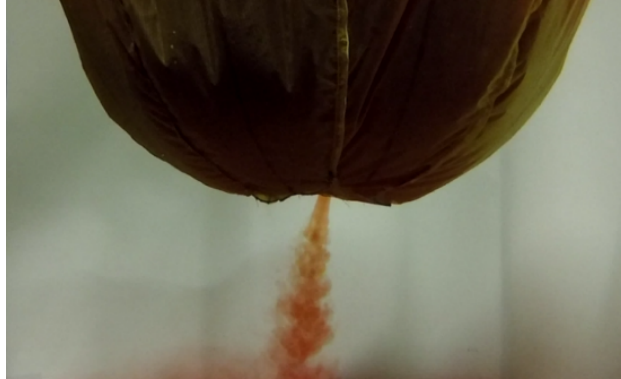
Figure 6: Snap-shot from test no. 8. Outflow appear as an axisymmetric turbulent jet. A small inclination angle of the discharged plume relative to the vertical was observed.
